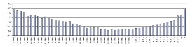
Typical self-noise of the microphone system when the microphone is substituted by a capacitor with similar capacitance as the microphone. Note that the acoustical self-noise for a real microphone will be higher due to thermal noise in the microphone cartridge.
