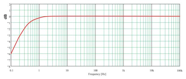
Typical frequency response for the preamplifier Nor1207. The combination of microphone and preamplifier has an additional typical attenuation of 6 dB relative to the open circuit sensitivity of the microphone.
