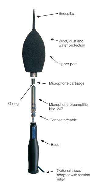
Screw the lock nut on the preamplifier onto the female connector on the cable. Push the preamplifier carefully into the base unit. The preamplifier and microphone is aligned in the correct position by a spring force. After mounting the upper protection part, the outdoor microphone unit will be ready for use. However, we recommend that you test the unit together with the measuring instrument by applying a calibrator before the upper part is mounted.
