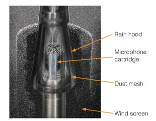
The typical frequency response for the preamplifier Nor1207 is shown below. The frequency response for the outdoor microphone system is therefore mainly determined by the microphone cartridge and the acoustic performance of the enclosure.
