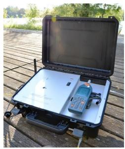
The measurement system is suitable for mounting indoors as well as outdoors and is easy to set up and operate: calibrate the microphone and start the measurement. A weather station can be included in the system.
