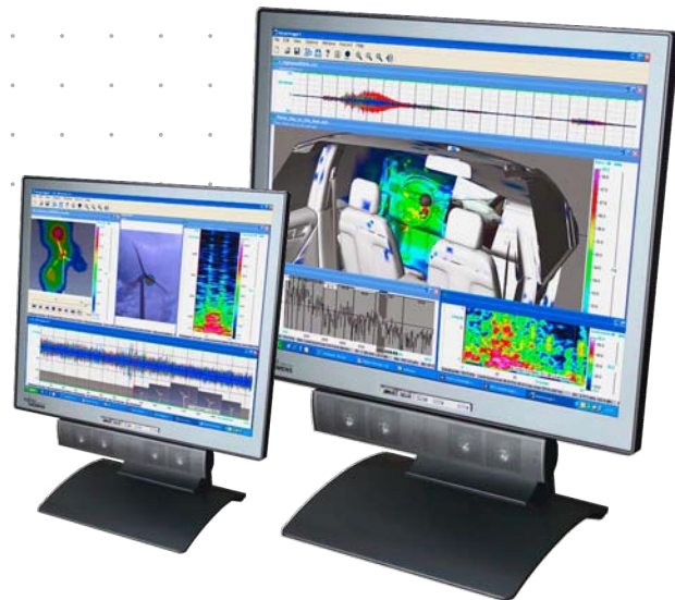
• • • Acoustic Movie 2D of a wind turbine and Acoustic Photo 3D of car interior including spectral analysis.
