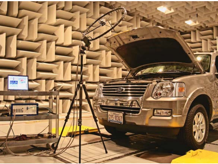
Above: Underhood measurement using Ring Array. Left: Acoustic Photo 3D of an engine.
