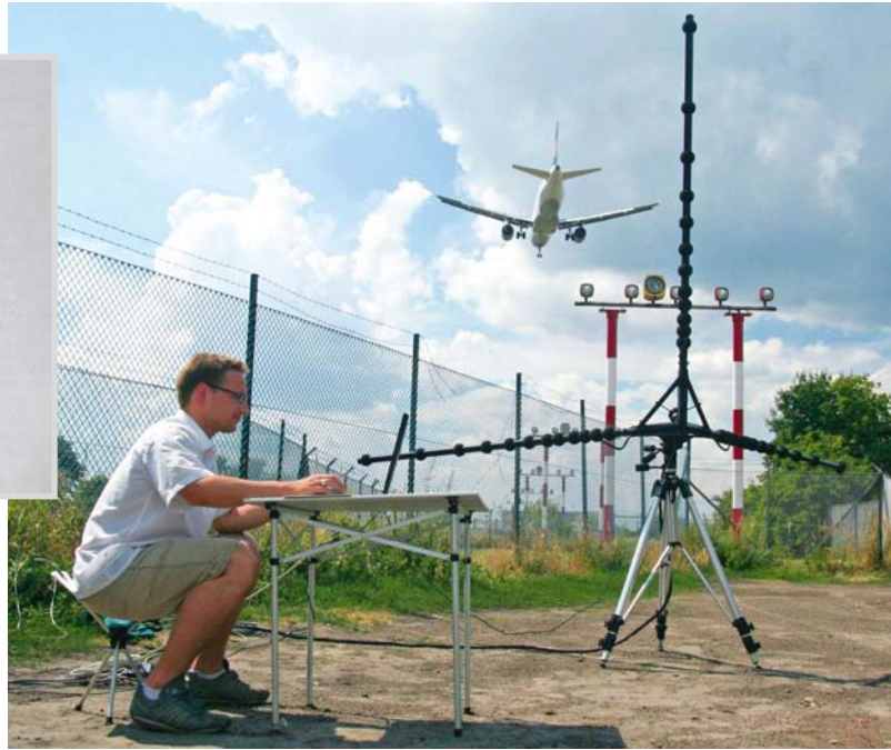
• • • Noise radiation from aircraft engines, gear and flaps and Acoustic Movie 2D.
