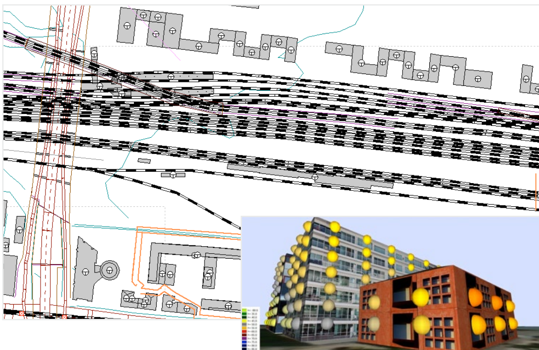
CadnaA 2D view of a railroad and road noise project and 3D View with Building Noise Map results
