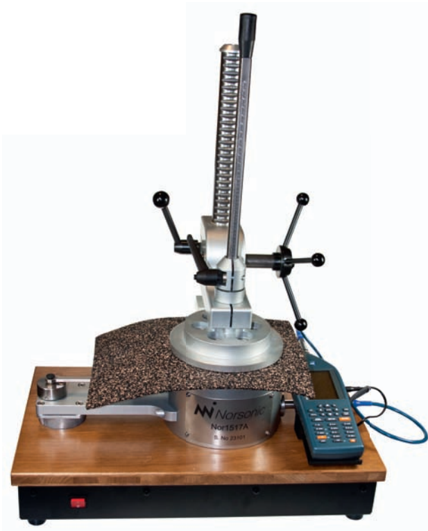
Thin specimen may be clamped between the test-vessel and the top.
