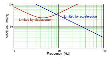
The lower limit is set by the noise floor in the transducer and measuring instrument. If the instrument has an electrical noise floor of 0,3  $\mu$ V – achievable for restricted frequency bands – this corresponds to a vibration level of 10<sup>-8</sup> m/s or 0,00001 mm/s with the nominal sensitivity of 26 Vs/m. The noise in the transducer itself is even lower – mainly determined by the source resistance of 380 ohm which corresponds to about 0,04  $\mu$ V in a bandwidth of 250 Hz.
