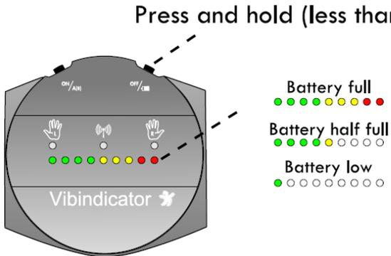
Figure21: Press and hold button2 to check battery status.
