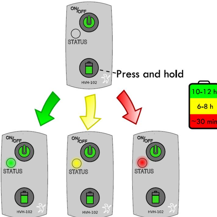
Figure 15: Press and hold down button 2 for battery status.
