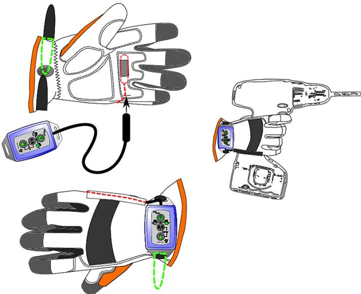
*Figure1: Place the sensor inside the palm. Mount the cable inside the canal. Fasten the analysis unit to the wrist.*
