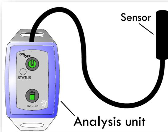
The HealthVib HAV Passive has two buttons and a LED for operating the unit.
