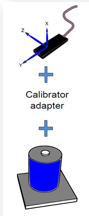
Figure36: Mounting the HealthVib HAv to the shaker for calibration
