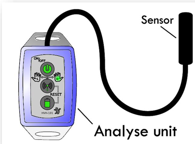
The HealthVib HAV Active has three buttons and two LED's for operating the unit.
