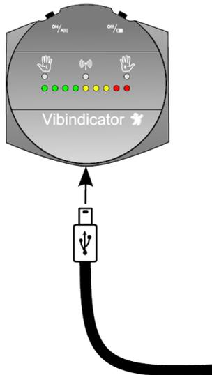
*Figure24: Insert USB-cable & connect it to charger.*
