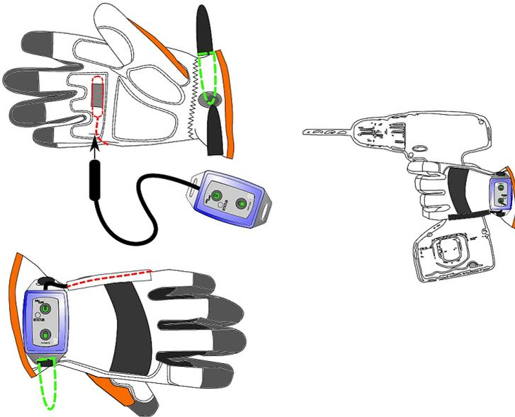
*Figure 11: Place the sensor inside the palm. Mount the cable inside the canal. Fasten the analysis unit to the wrist.*
