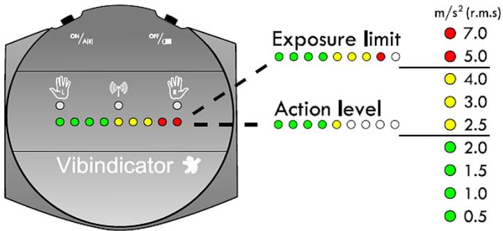
Figure 19: Vibration level is displayed as color and number of LED's.
