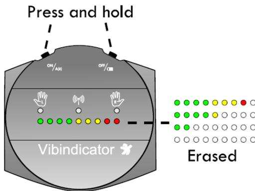
*Figure22: Press & hold both left & right button until the LED's are turned off.*
