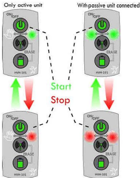
Figure 4: Press button 1 to start and stop measurement
