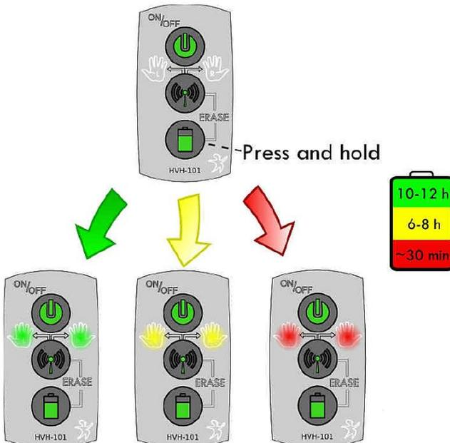
Figure 6: Press button 3 to see battery status. The LED's will turn green, yellow or red.
