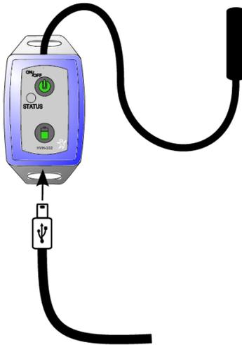
*Figure 17: Connect USB-cable to unit and charger to wall socket.*
