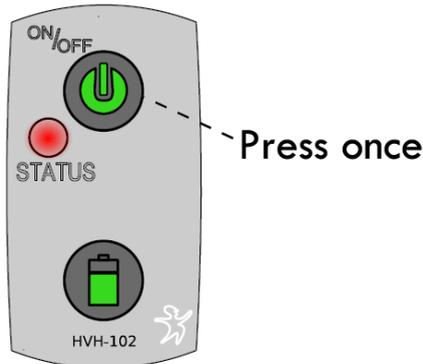
*Figure 13: Turn on the unit by pressing button 1*
