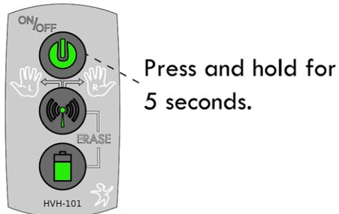
*Figure 7: Press and hold button 1 for 5 seconds.*
