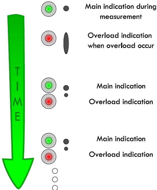
Figure 14: Overload is indicated by flashing after the main indication (either measurement or paused mode.)
