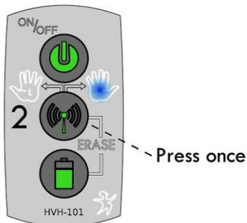
Figure 3: Press button 2 to start searching for other units.
