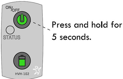
*Figure 16: Press and hold button 1 for 5 seconds.*
