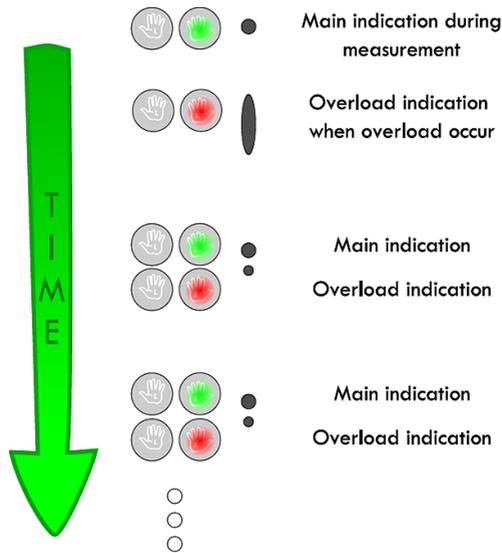
Figure 5: Overload is indicated by flashing red shortly after the main indication of measurement or paused.
