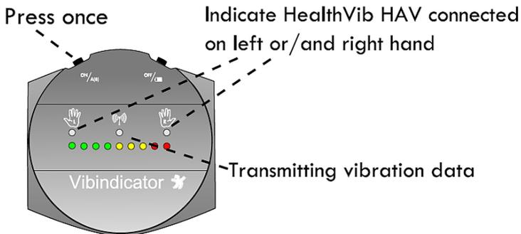
*Figure 18: Press button 1 to start the unit.*
