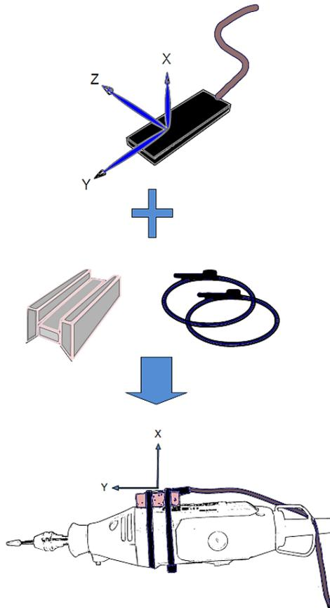
*Figure 12: Example of alternative (Adaptor + machine) mounting.*
